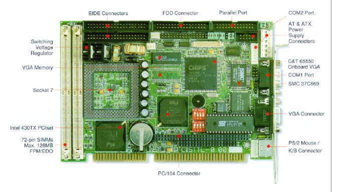
Intel Pentium or K6 processors up to 266 MHz Intel 430TX PCIset 512K synchronous Pipeline Burst cache On-board PCI Flat Panel VGA controller Ultra DMA/33 IDE controller ACPI (Advanced Configuration Power Interface) Support 0° to +60° C operation temperature range
