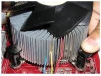
8.Engage the fasteners caps. Apply thumb pressure to the top of each of the 4 fastener caps, there is no specific order of engagement, you will hear a "click" upon full engagement.
