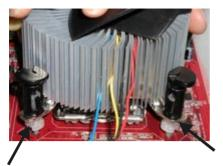
7. Align the fastener tips with the motherboard hole pattern, insert the fastener tips into the holes, guiding the wires to avoid pinching. The fasteners will slide through the motherboard holes with no insertion force.
