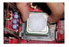
3.Use index finger and thumb to place the CPU onto the plastic body (look for the gold arrow on the CPU. The gold arrow should point away from the lever pivot).
