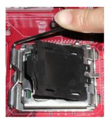
4.Use index finger and thumb to press down metal lever, the cap will be pushed up by the CPU; this may also be done by removing the cap beforehand.
