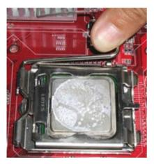
5.Press the metal lever so it is secured in the bottom steel shell grip hook.
