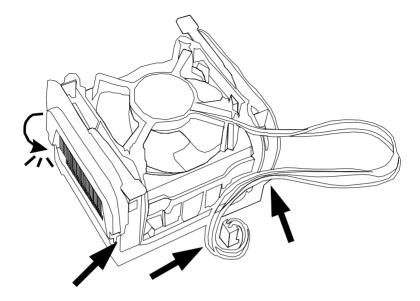
6. Use one end of the clip to hook the latch of the CPU sliding plate and then hook the other three latch to fix the cooling fan set. At last, connect the fan to the power supply connector provided on your mainboard.
