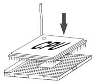
3. If the CPU is correctly installed, the pins should be completely embedded into the socket and can not be seen. Please note that any violation of the correct installation procedures may cause permanent damages to your mainboard.
