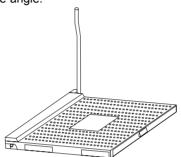
2. Look for the gold arrow. The gold arrow should point towards the lever pivot. The CPU can only fit in the correct orientation.
