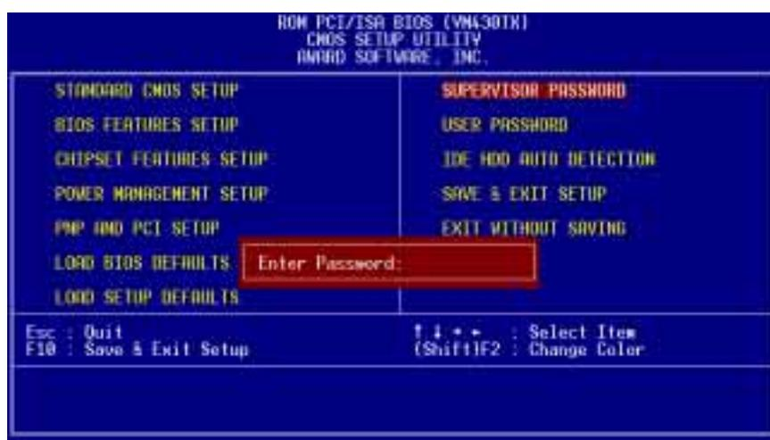
To implement password protection, specify under “Security Option” in the BIOS Features Setup screen when the system will prompt for the password. To disable either password, press <Enter> instead of entering a new password when the “Enter Password” prompt appears. A message confirms that the password has been disabled.
