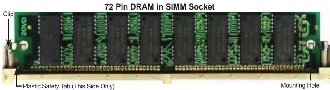
To release the memory module, squeeze both metal clips outward and rock the module out of the metal clips.
