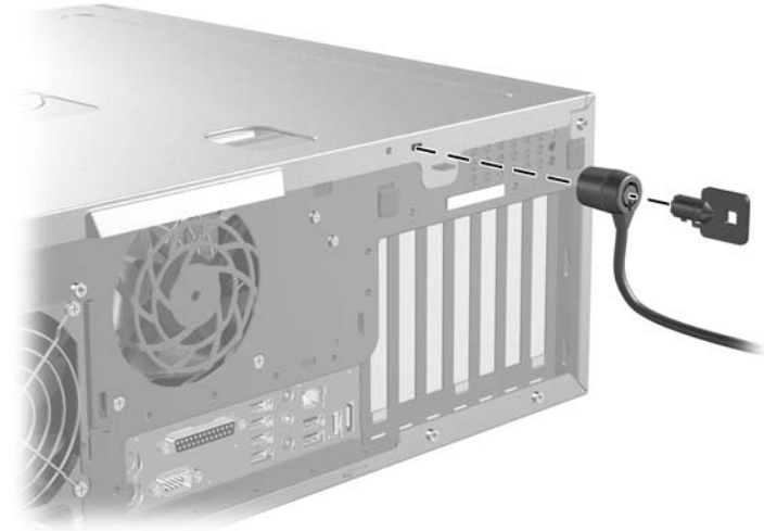
Figure 4-4 Removing the cable lock
