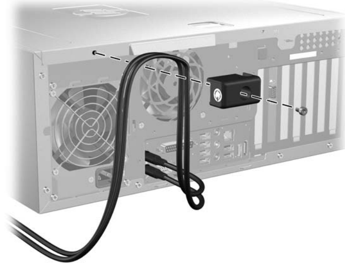
Figure 4-6 Removing the lock screws
