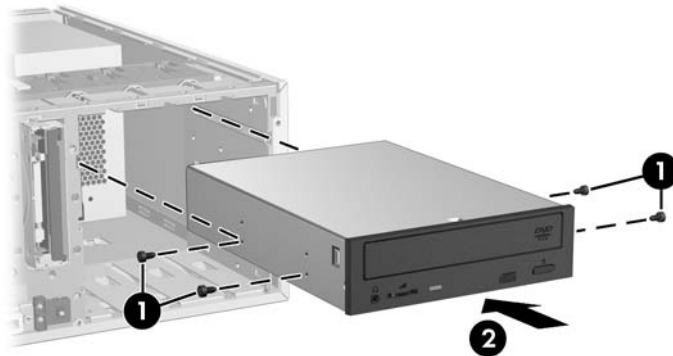
Figure 4-44 Installing the optical drive
