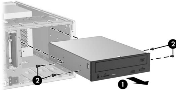
Figure 4-43 Removing the optical drive screws
