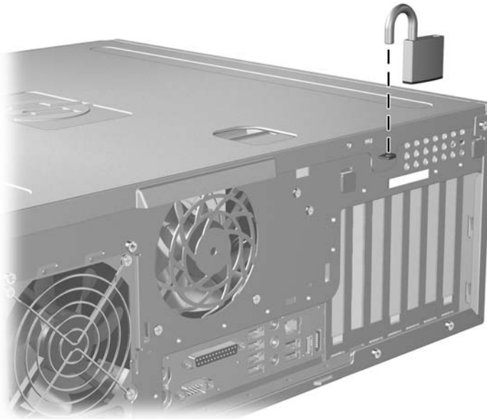
Figure 4-3 Removing the security lock
