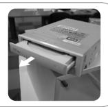
Plip down the Optical drive and remove the bezel from the disk tray.
