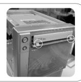
Please disassemble your optical drive first. On the bottom of the disc try there is a tiny hole. Gently poke the hole with a needle to eject the Disk Tray.
