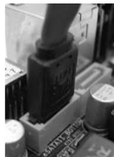
Connect the SATA data cable to one of the orange eSATAII connector (eSATAII_BOTTOM)
