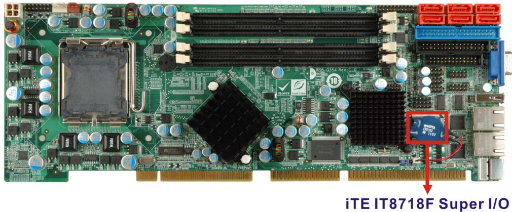
Figure 2-13: ITE IT8718F Super I/O
