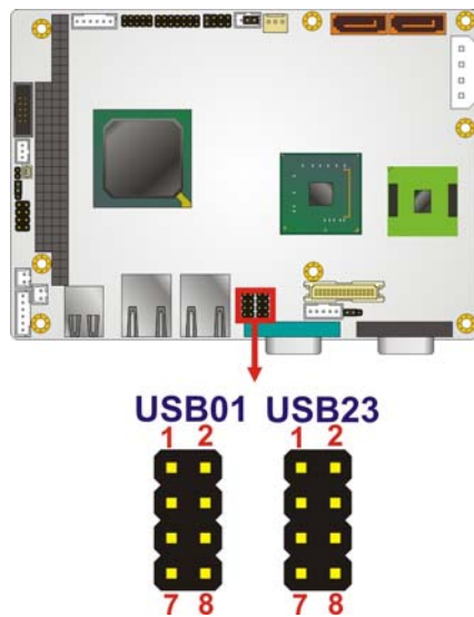
Figure 3-21: USB Connector Pinout Locations
