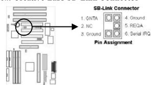
Connect an optional Creative Labs PCI sound card to this 5-pin connector. This connector is necessary for migrating the legacy Sound Blastercompatible audio to the PCI bus.
