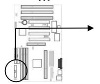
Connect the single end of a floppy disk drive cable to this 34-pin connector block. Connect the other ends of the cable to one or more floppy disk drives. The connector with twisted wires always connects to drive A; the connector without twisted wires connects to drive B.
