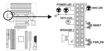
The J1 connector actually consists of five connectors for the speaker, switches, and LED indicators on the front panel.
