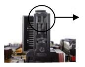
3. If you are installing a SECC type CPU, make sure the CPU is secured in place by pushing the locks outward so that the lock shows through the retention mechanism's lock holes.
