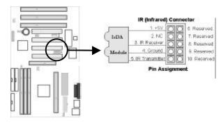
This 5-pin connector supports an optional wireless transmitting and receiving infrared module. This module mounts to a small opening on system cases that support this feature. Connect a ribbon cable from the module to the connector according to the pin definitions.
