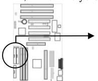
These connectors support IDE hard disk and CD-ROM drives. After connecting the single end of the provided IDE ribbon cable to the board, connect the two plugs at the other end to your hard disk or CD-ROM drives.
