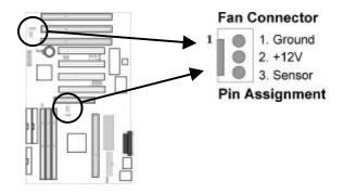
These 3-pin connectors support fans of 12V DC/500mA (6W) or less with a minimum of 3.500RPM.
