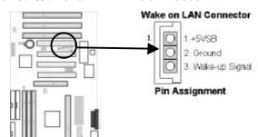
This 3-pin connector allows the system to power up when a wakeup signal is received from the network through an optional LAN card (with remote wakeup capabilities).
