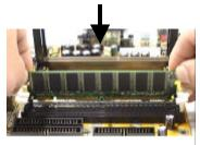
To insert a DIMM, align the module with the socket key and press down until the levers at each end of the socket snap closed.
