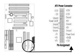
This 20-pin connector connects to an ATX power supply. Find the correct orientation and push the plug down firmly, making sure the pins are aligned. (Due to different hole sizes, you can insert the plug in only one orientation.)
