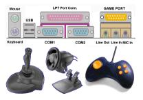
You can connect your joystick, game pad, or other simulation hardware device DIN 15pin plugs to this connector. Please refer to the further connection notes of the device's user's manual for further detailed information.
