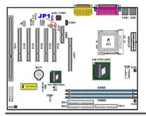
This header can select whether the AMR card insertion on the AMR slot is primary or secondary. When you don't want to use the onboard audio CODEC, you have to set JP1 at open. The default setting is short. Remember that only when using an MC 97 card should you select the JP1 as open. Otherwise, leave it selected as short.
