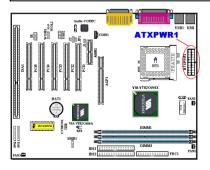
Attach the connector from the power supply to the ATXPWR1 connector here. Remember you have to push the connector from the ATX power supply firmly to the end with the ATXPWR1 connector, insuring that you have a good connection.
