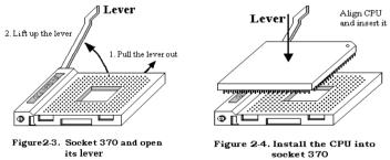
When you raise the lever, you have to loosen the socket lock. Please raise the lever to the end, and prepare to insert the processor. Next, you need to align the processor pin 1 to the socket pin 1. If you put it in the wrong direction, you will not be able to insert the processor easily, and processor pins will not fully go into the socket. If that is the case, please change the direction, until it easily and fully inserts into the 370 socket. See Figure 2-4.
