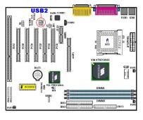
This header is for connecting the additional USB ports plugs. You can use the special USB port expend cable (option), it can provides you additional two USB plugs, you can fix these USB plugs on the back panel.
