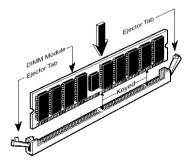
Figure 2-6. Memory module installation
