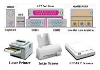
This parallel port is also called an "LPT" port, because it usually connects to the printer. You can connect other devices that support this communication protocol, like an EPP/ECP scanner, etc.
