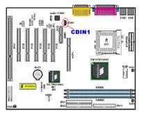
This header is for the internal CD-ROM drive audio cable connection use, and this header are used for specify type of CD audio cable connector. Please check your audio cable attached with the CD-ROM drive to see which type connector you have, then plug it to this header.
