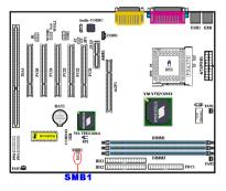
This connector is reserved for system management bus (SM bus). The SM bus is a specific implementation of an  $l^2C$  bus.  $l^2C$  is a multi-master bus, which means that multiple chips can be connected to the same bus and each one can act as a master by initiating a data transfer. If more than one master simultaneously tries to control the bus, an arbitration procedure decides which master gets priority.
