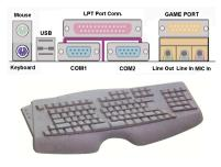
Attach a PS/2 keyboard connector to this 6pin Din-connector. If you use an AT keyboard, you can go to a computer store to purchase an AT to ATX converter adapter, then you can connect your AT keyboard to this connector. We suggest you use a PS/2 keyboard for best compatibility.
