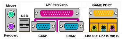
Figure 2-13. VL6 back panel connectors
