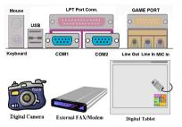
This motherboard provides two COM ports, you can connect an external modem, mouse or other devices that support this communication protocol to these connectors.
