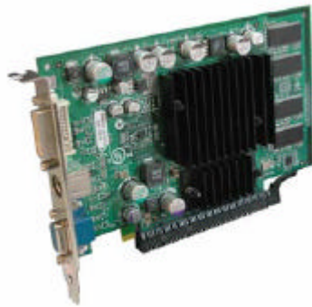
Figure 31: Install a PCI Express x16 card
