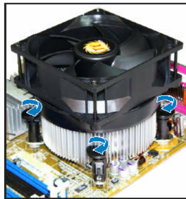
Figure 23: Rotating the Push-Pins
