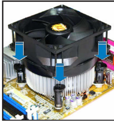
Figure 22: Securing the Heatsink
