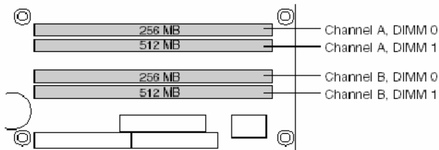
Figure 27: Dual Channel Mode Configuration with Four DIMMs
