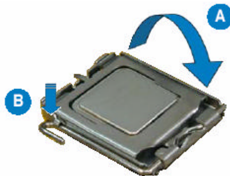
Figure 20: Closing the Load Plate
