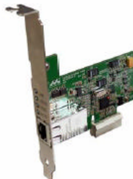
Figure 32: Install a PCI Express x1 card
