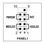
Figure 5: Front Panel connectors
