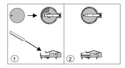
Figure 10: Removing the Battery
