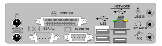
Figure 2: Rear I/O Shield
