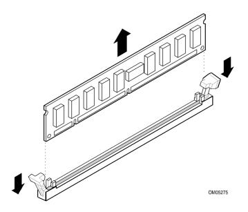
Figure 7: Removing Memory Modules
