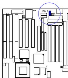
**CPU Fan Connector: CPU\_FAN**
