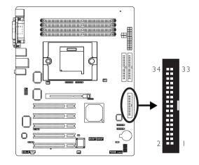
The system board is equipped with a shrouded floppy disk drive connector for connecting two standard floppy disk drives. To prevent improper floppy cable installation, the shrouded floppy disk header has a keying mechanism. The 34-pin connector on the floppy cable can be placed into the header only if pin I of the connector is aligned with pin I of the header.
