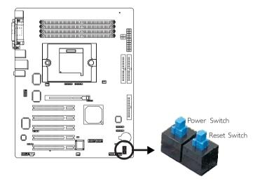
The presence of the power switch and reset switch on the system board are user-friendly especially to DIY users. They provide convenience in powering on and/or resetting the system while fine tuning the system board before it is installed into the system chassis.
