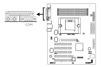
The system board is equipped with an onboard serial port (Teal/ Turquoise) at location J1. The serial port is an RS-232C asynchronous communication port with 16C550A-compatible UARTs that can be used with a modem, serial printer, remote display terminal or other serial devices.
