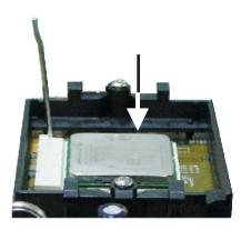
7. Once the CPU is in place, push down the lever to lock the socket. The lever should click on the side tab to indicate that the CPU is completely secured in the socket.
