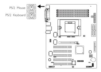
The system board is equipped with an onboard PS/2 mouse (Green) and PS/2 keyboard (Purple) ports - both at location CN2 of the system board. The PS/2 mouse port uses IRQ12. If a mouse is not connected to this port, the system will reserve IRQ12 for other expansion cards.
