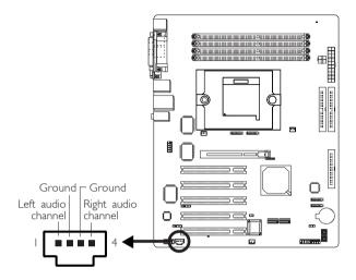
The CD-in (J4) connector is used to receive audio from a CD-ROM drive, TV tuner or MPEG card.
