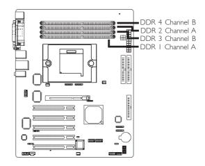
The system board supports DDR SDRAM DIMM. Double Data Rate SDRAM (DDR SDRAM) is a type of SDRAM that doubles the data rate through reading and writing at both the rising and falling edge of each clock. This effectively doubles the speed of operation therefore doubling the speed of data transfer. Refer to chapter I (System Memory section) for detailed specification of the memory supported by the system board.
