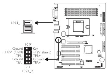
The system board is equipped with an onboard IEEE 1394 port at location CN3 (IEEE 1394\_1) of the system board.
