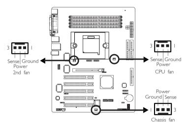
Connect the CPU fan's cable connector to the CPU fan connector (J32) on the system board. The 2nd fan connector (J6) and chassis fan connector (J31) are used to connect additional cooling fans. The cooling fans will provide adequate airflow throughout the chassis to prevent overheating the CPU and system board components.
