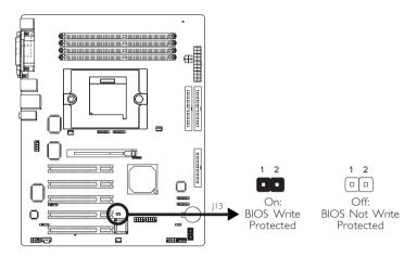
JI3 is used to enable or disable the BIOS Write Protect function. When enabled, the system will be protected from unnecessary updating or flashing of the BIOS. It secures the BIOS therefore any updates to it will not take effect.
