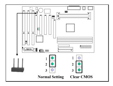
Note: Improper BIOS setting may cause hang-up to the PC system, Should it be happened, you can use JP4 to clear the information which is stored in the CMOS memory and get the PC system back to normal. Improper connection may cause permanent damage to the mainboard. Please refer to the following steps to clear the CMOS
