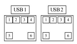
Pin1: +5VDC Pin2: DATA-Pin3: DATA+ Pin4: Ground Pin5: Ground Pin6: Ground
