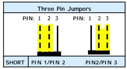
If you have made an improper setting in the BIOS setup and your computer is not functioning, or if you have forgotten your password, you can use this jumper, JP 9, to clear the CMOS memory and to reconfigure your system.
