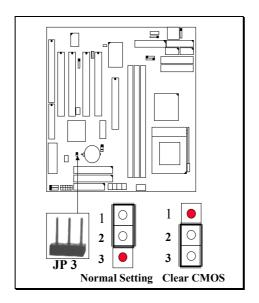
Note: Improper BIOS setting may cause hang-up to the PC system, In case that it should be happened, you may use JP3 to clear the CMOS memory and get the PC system back to normal. Please refer to the following steps to clear the CMOS
