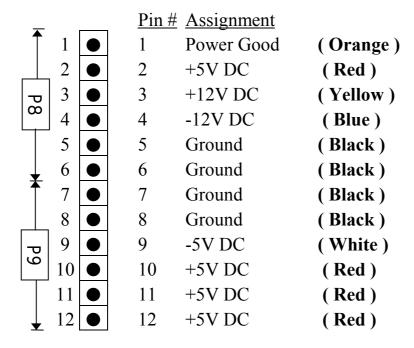
Note: There are two connectors from the switching power supply (P8 & P9), Wrong connection will cause permanent damage to the mainboard. Be sure to make the power connector correctly all the time. Joint the black cable and then have the connectors connected to the mainboard.
