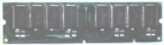
Picture of DIMM module
