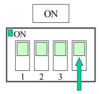
Push the switch upward to select "ON"
