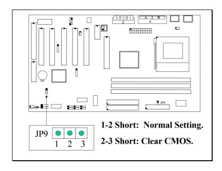
Followings are the procedures to use JP9 to clear the BIOS setting which is saved in the CMOS memory.
