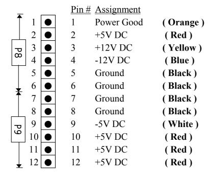
Note: There are two connectors from the switching power supply (P8 & P9), Wrong connection will cause permanent damage to the mainboard. Be sure to make the power connector correctly all the time. Joint the black cable and then have the connectors connected to the mainboard.
