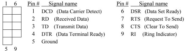
I/O address 3F8H/2F8H/3E8H/2E8H, IRQ3/IRQ4, selected by CMOS setup.
