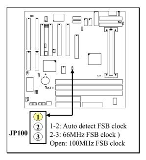
(When select 1-2 setting, the system board will detect the FSB clock automatically.) (When select 2-3 setting, the FSB clock will be always 66MHz despite of CPU type.) (When no jumper on JP100, FSB clock will be always 100MHz despite of CPU type)
