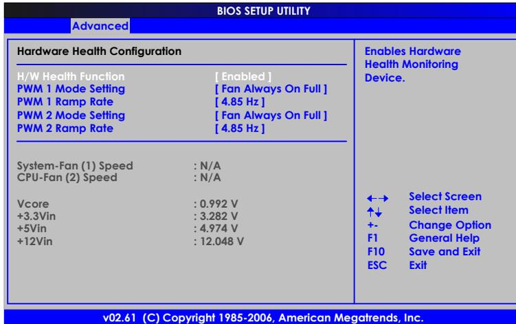
The PC Health Status displays the current status of all of the monitored hardware devices/components such as CPU voltages, temperatures and fan speeds.
