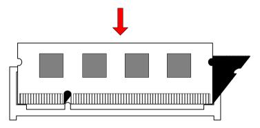
Push the SODIMM module back towards the board until the clips lock the module in place.
