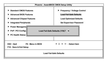
This option is for restoring all the default fail-safe BIOS settings. These values are set by the mainboard manufacturer to provide a stable system with basic performance.
