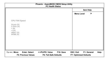
The PC Health Status displays the current status of all of the monitored hardware devices/components such as CPU voltages and fan speeds.
