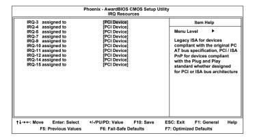
**NOTE:** The items are adjustable only when "Resources Controlled By" is set to "Manual".
