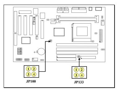
This mainboard is designed by using either VIA 693 or 693A chipset. When VIA693 is installed on the mainboard, you will see only JP100 on the board and you can use it to tell the mainboard to use the choosen FSB clock in the following table despite the CPU installed on the mainboard. If you found the VIA693A chipset installed on the mainboard, then you will see both JP100 and JP133 on the board and you can refer to the following table to select different FSB clock:
