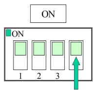
Push the switch downward to select "OFF" Push the switch upward to select "ON"
