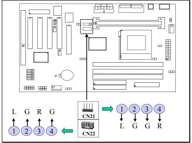
Note: L = Left channel audio-out R = Right channel audio-out G = Audio Ground
