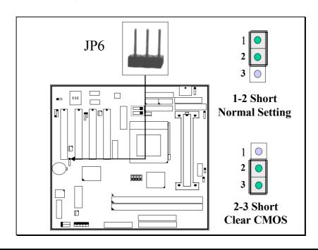
Note: Improper BIOS setting may cause hang-up to the PC system, Should it be happened, you may use JP6 to clear the information which is stored in the CMOS memory and get the PC system back to normal. Improper connection may cause permanent damage to the mainboard. Please refer to the following steps to clear the CMOS
