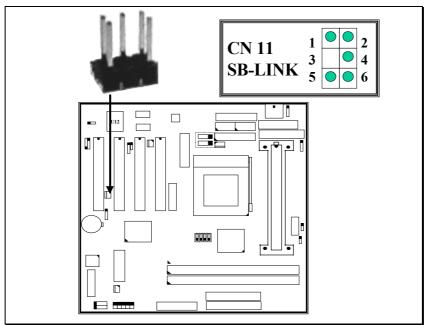
(SB-Link is designed for PCI sound cards such as Creative<sup>TM</sup> EMU8008 sound chip)
