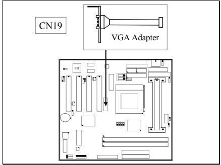
The VGA connector on the board is the AGP VGA interface and you can use an adapter as shown in the above picture to connect it to your VGA monitor.
