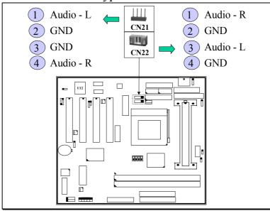
Note: Audio - L = Left channel audio-out Audio - R = Right channel audio-out
