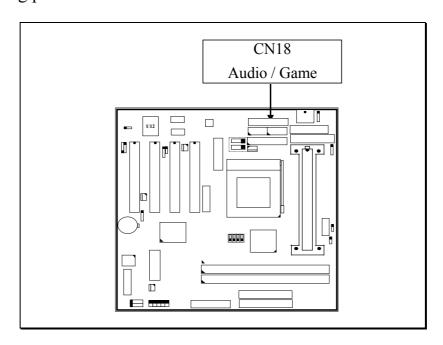
In order to have the audio device connected to the Audio Game port, an adapter is required. Please refer to the following picture for the connections on the adapter
