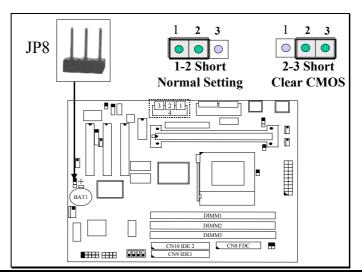
Note: Improper BIOS setting may cause hang-up to the PC system, Should it be happened, you may use JP8 to clear the information which is stored in the CMOS memory and get the PC system back to normal. Improper connection may cause permanent damage to the mainboard. Please refer to the following steps to clear the CMOS
