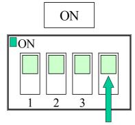
Push the switch upward to select "ON"
