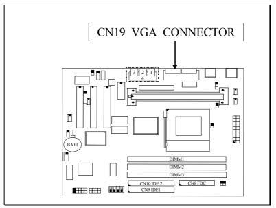
The VGA connector on the board is the AGP VGA interface and you can connect it direct to your VGA monitor.
