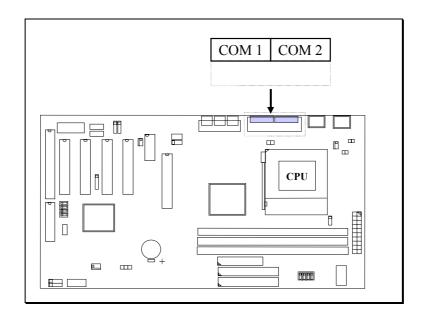
(I/O address: 3F8H/2F8H/3E8H/2E8H, IRQ3/IRQ4, selected by CMOS setup.)
