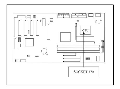
Be sure to remove the power cable from the PC system when installing CPU or any other components.
