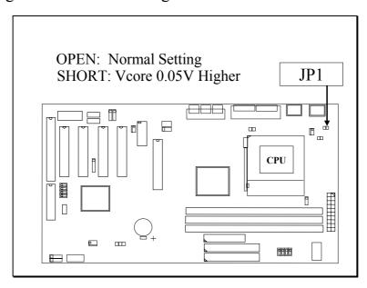
Note: When you use JP1 to raise the CPU voltage, it does not mean that CPU over clock is guaranteed!.
