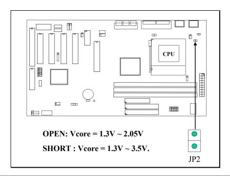
When JP2 is not installed on the mainboard, it will support Vcore between 1.3V and 2.05V.
