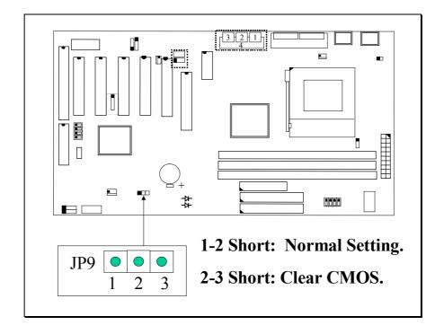
Basically, the BIOS setup program will have all the setting saved in the CMOS memory which is included in the core logic of the mainboard. If you want to clear the setting which is saved in the CMOS memory, you may use JP9 and refer to the following procedure to clear the information in the CMOS.
