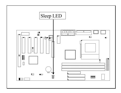
Sleep LED is designed to indicate the status of the PC system. When the PC system is powered on, the sleep LED will be darkened. When the power of the PC system is OFF, the sleep LED will be lightened to indicate the PC system is now under sleep mode.
