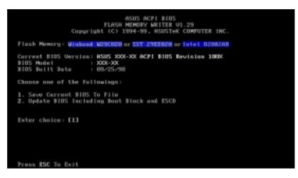
**IMPORTANT!** If the word "unknown" appears after **Flash Memory:**, the memory chip is either not programmable or is not supported by the ACPI BIOS and therefore, cannot be programmed by the Flash Memory Writer utility.
