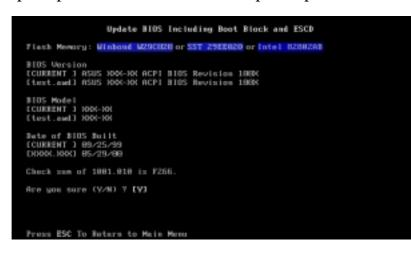
7. The utility starts to program the new BIOS information into the Flash ROM. The boot block is updated automatically only when necessary. This minimizes the possibilities of boot problems in case of update failures. When the programming is done, *Flashed Successfully* appears.
