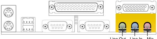
Line Out Line In Mic 1/8" Stereo Audio Connectors
