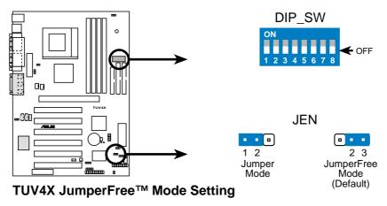
**NOTE:** In JumperFree<sup>™</sup> mode, set all DIP switches (DIP\_SW) to OFF.
