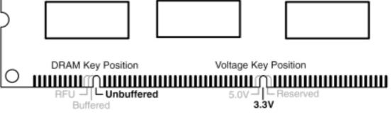
The notches on the DIMM shifts between left, center, or right to identify the type and also to prevent the wrong type from being inserted into the DIMM slot on the motherboard. You must tell your retailer the correct DIMM type before purchasing. This motherboard supports four clock signals per DIMM.
