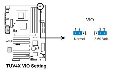
**WARNING!** Using a higher voltage may help when overclocking the system but it may shorten the life of system components. As much as possible, keep the VIO jumper to its default setting for better system stability.
