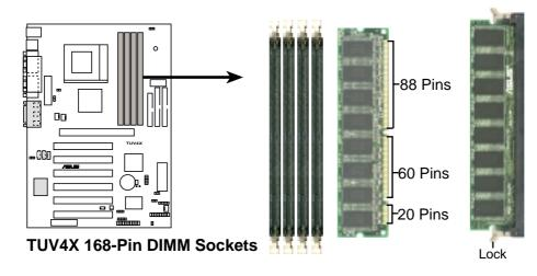
The DIMMs must be 3.3Volt unbuffered SDRAMs. To determine the DIMM type, check the notches on the DIMMs (see the figure below).
