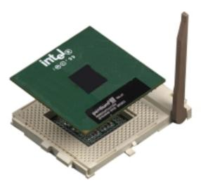
**CAUTION!** The CPU fits only in one orientation. Do not force the CPU into the socket to prevent bending the pins and damaging the CPU. If the CPU does not fit completely, check its orientation or check for bent pins.
