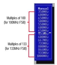
**CPU : System Frequency Multiple (when CPU Speed is set to [Manual])** This field is for unlocked processors only. If your processor frequency multiple is detected locked, you cannot access this field. This field sets the frequency multiple between the CPU's *internal* frequency (CPU speed) and *external* frequency. Set this field in conjunction with **System/PCI Frequency** (**MHz**) to match the speed of the CPU. Configuration options: [2.0x] [2.5x] [3.0x]...[7.0x] [7.5x] [8.0x]
