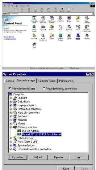
2. Under System Properties, click on the Device Manager tab. Double click on Realtek 8129 PCI Fast Ethernet. Click the Driver tab as shown. Now click the Update Driver button.
