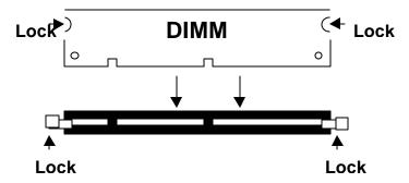
**Top View of DIMM Socket**
