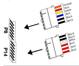
**Power Connector Keys** The power connectors are keyed to prevent incorrect installation. The connector keys must be cut to fit some power supplies, as shown below.
