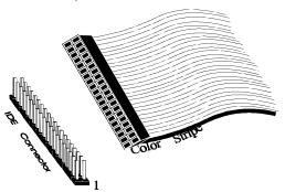
P1 is a 40-pin dual-inline berg that connects an IDE drive to the primary onboard IDE connector. This motherboard supports IDE Modes 0, 1, 2, 3, and 4, IDE prefetch, LBA (Logical Block Address) mode, high capacity drives (over 528 MB), 32-bit data transfer, and fast IDE transfer. These IDE features are configured in Peripheral Setup in the WINBIOS Setup utility.
