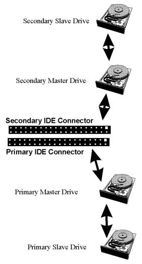
**Attach IDE Cable** P1 is the primary IDE (Integrated Drive Electronics) hard disk drive connector. Both the primary master and the primary slave IDE drives must be connected by cable to P1, as shown below.
