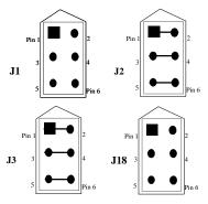
**From 3.3V Power Supply** Set J1, J2, J3, and J18 as follows to configure 3.3V power from the 3.3V power supply:
