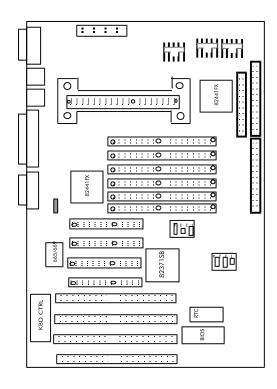
Figure 1: Layout of the TI6NFK motherboard, Klamath processor and KP6
