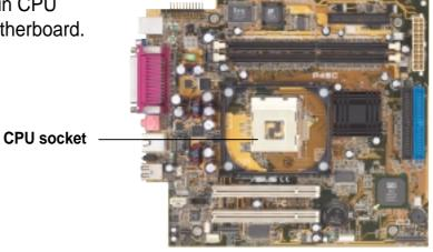
2. Unlock the socket by pressing the lever sideways then lifting it up to a 90°-100° angle.
