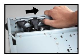
4. Unlatch the drive frame by pulling it outward.
