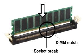
Firmly insert the DIMM into the socket until the retaining clips snap back in place and the DIMM is properly seated.
