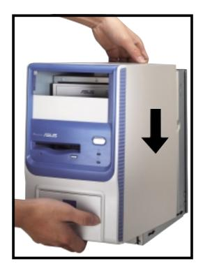
5. Fit the rail tabs on the sides and bottom of the cover to the edges of the chassis.
