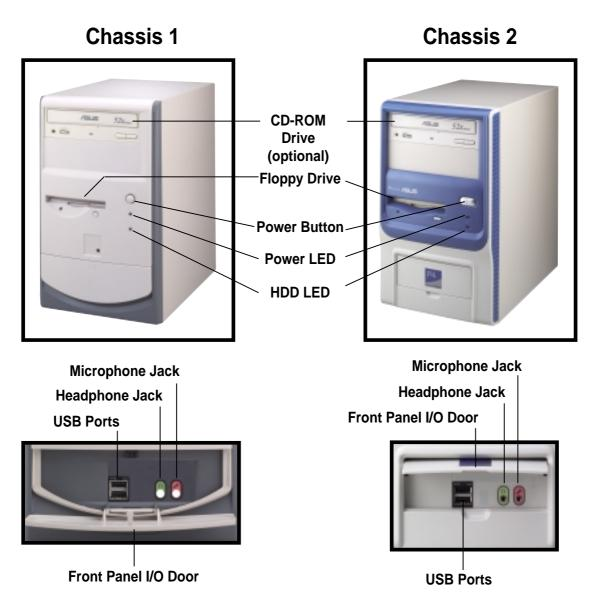
The lower part of the front panel is a door that covers accessible I/O features including two USB ports (Ports 2&3), a headphone jack, and a microphone jack.
