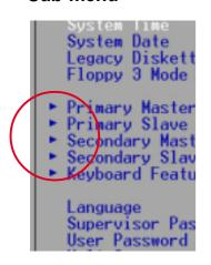
Note that a right pointer symbol (as shown on the left) appears to the left of certain fields. This pointer indicates that you can display a sub-menu from this field. A sub-menu contains additional options for a field parameter. To display a sub-menu, move the highlight to the field and press <Enter>. The sub-menu appears. Use the legend keys to enter values and move from field to field within a sub-menu as you would within a menu. Use the <Esc> key to return to the main menu.
