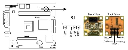
**P4SC Infrared Module Connector**
