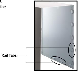
6. Push the cover towards the rear until it fits. The locking tab snaps into the hole on the chassis indicating that the cover is in place.
