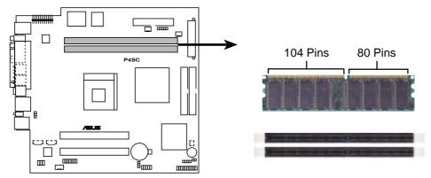
P4SC 184-Pin DDR DIMM Sockets
