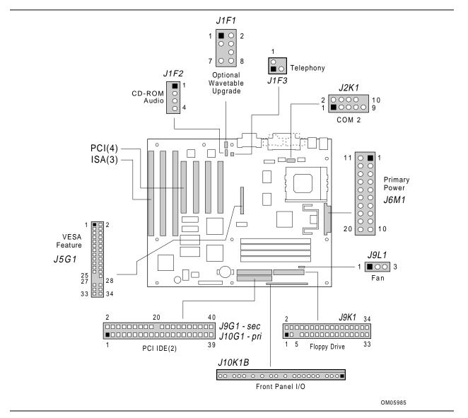
Figure 3. Motherboard Connector Locations
