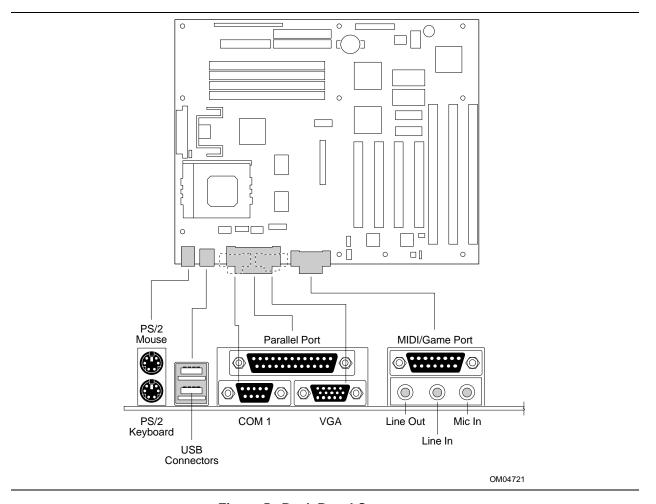
Figure 5. Back Panel Connectors
