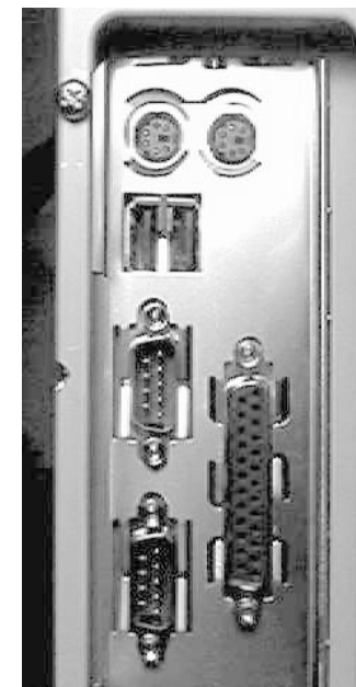
I/O connector aligned with openings
