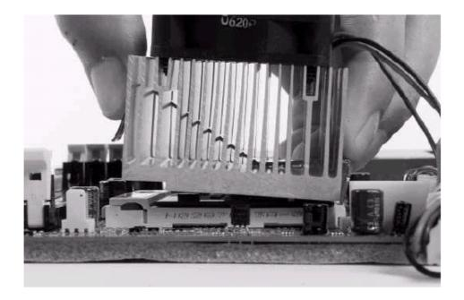
3. To install this clip, push firmly only on the end of the clip. To install the clip, typically requires 12 to 24 pounds of force.
