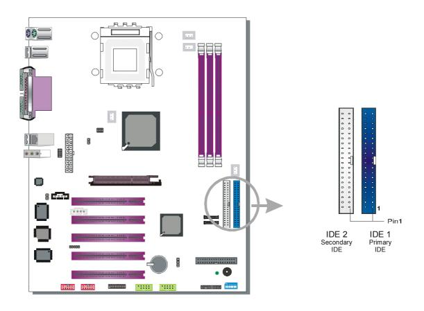
This motherboard offers two primary and two secondary IDE device connectors (IDE1, IDE2), can support up to four high-speed Ultra DMA 33/66/100/133 HDD or CD-ROM. SATA1/2 can support up to 4 ATA 150 SATA hard disks..IDE1,2/ SATA1,2 are controlled by the 8237 South bridge chip.
