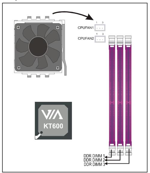
**Note:** If the fan is defective or Power connector is not connected to CPUFAN1, the system will enable Fan Off Control function. See below for more information on FOC function.
