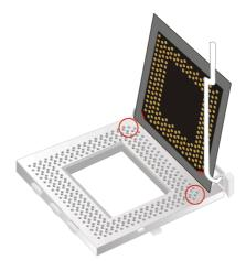
3. Seat the processor in the socket completely and without forcing.
