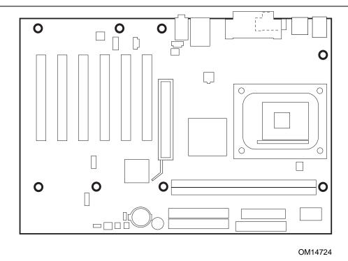
Figure 4. Desktop Board Mounting Holes
