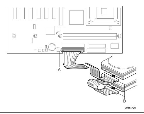
Figure 9. Connecting the IDE Cable
