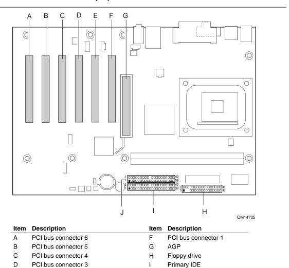
Figure 16. Add-in Card and Peripheral Interface Connectors
