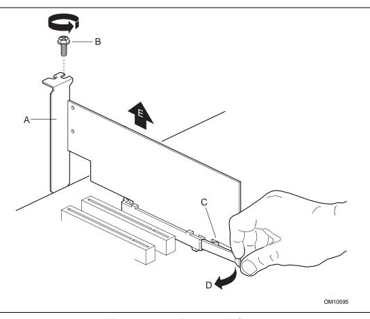
Figure 8. Removing the AGP Card
