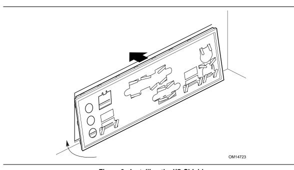
Figure 3. Installing the I/O Shield
