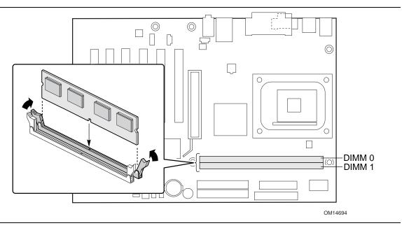
Figure 7. Installing a Memory Module
