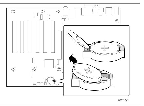
Figure 13. Removing the Battery
