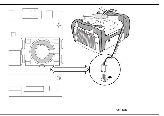
Figure 6. Connecting the Processor Fan Heat Sink Cable to the Processor Fan Connector
