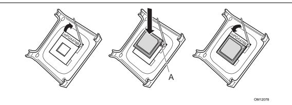
Figure 5. Installing a Processor
