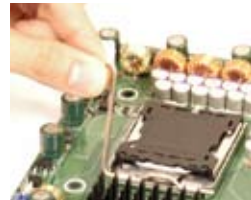
Load Lever CPU in the CPU socket
