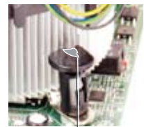
Narrow end of the groove points outward
