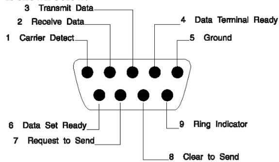
The DB9 serial port pinout is shown below.
