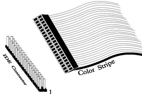
When you use the onboard IDE controller in conjunction with another hard drive controller, you must make sure that there are no conflicts in IRQ and I/O port addresses. The onboard IDE uses IRQ14 and I/O port addresses 01F0h – 01F7h. If there is a conflict, the IDE interface can be disabled via Peripheral Setup (see page 164). The J4 pinout is:
