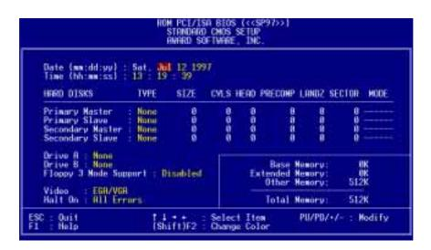
User-configurable fields appear in a different color. If you need information on the selected field, press <F1>. The help menu will then appear to provide you with the information you need. The memory display at the lower right-hand side of the screen is read-only and automatically adjusts accordingly.
