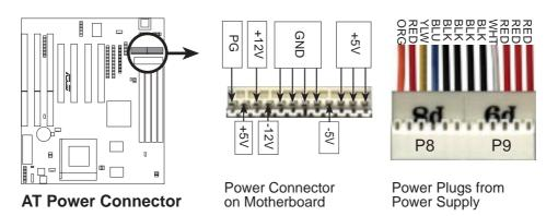
Using a slight angle, align the plastic guide pins on the lead to their receptacles on the connector. Once aligned, press the lead onto the connector until the lead locks into place.
