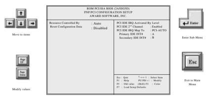
Figure 6: PNP/PCI Configuration Setup Menu
