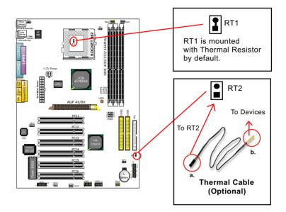
2-8.9 Thermal Connector and Thermal Resistor
