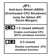
JP1 is designed to enable the overheat safeguard for some CPUs which are incorporated with a protective thermal diode. <u>The latest AMD Athlon XP and Duron Morgan CPUs are incorporated with such thermal diode and can be protected by this function.</u> Setting JP1 1-2 closed (default setting) will get system shutdown when the above-mentioned CPUs get to 85°C (the default protection temperature.) Only when the CPU returns to a cooler state can you restart your system.
