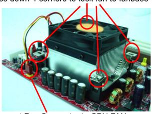
Connect Fan Connector to CPU FAN connector
