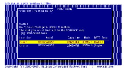
Next, you will see a message "Duplicate the SOURCE(Disk x) data to RAID disks?". Press <N> and <Enter> to create RAID 1 array only or press <Y> and <Enter> to duplicate the data from source disk to mirror disk.
