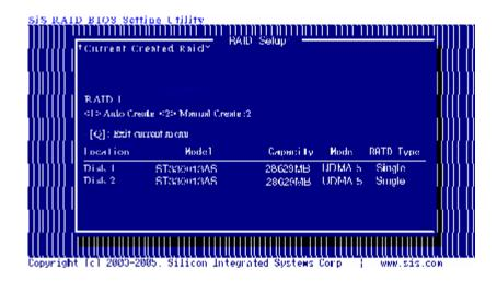
4. Use < ↑ > < ↓ > to select disk , and press <Enter> to select disk, <Q> to exit. When you press <Enter> on the disk you wanted, the RAID Type will be changed from Single to RAID 1. The same as RAID 0, the disk you select first will be the SOURCE disk.
