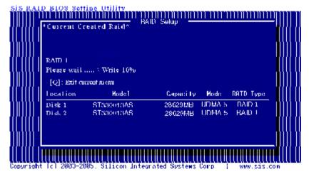
After all steps finished, press <Q> until escape the setup menu and RAID 1 array will be shown on the top of the main frame.
