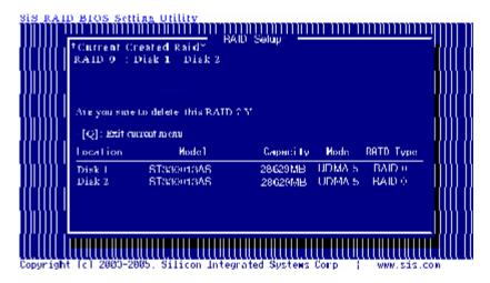
Press <Y> and <Enter>, the deleting action finish. And the RAID Type of all disk members of this RAID array will be changed from RAID 0 to Single.
