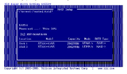
After all steps finished, press <Q> until escape the setup menu and RAID 0 array will be shown on the top of the main frame.
