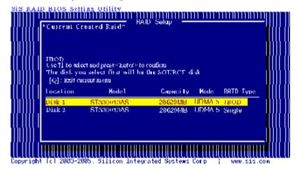
5. After all steps finished, press <Q> until escape the setup menu and JBOD array will be shown on the top of the main frame.
