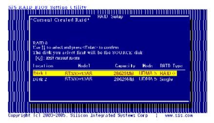
Next, you will see a message "Split the SOURCE(Disk x) data to RAID disks?". Press <N> and <Enter> to create RAID 0 array only or press <Y> and <Enter> to split the data from source disk to other disks.
