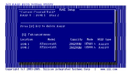
2. Press <D> to start deleting a RAID array.
