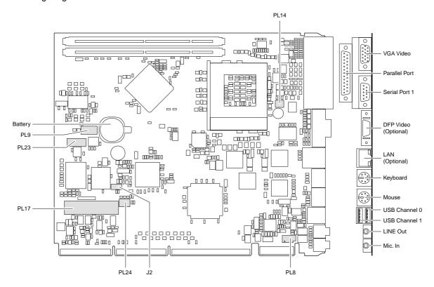
**NOTE:** The Mouse and Keyboard are interchangeable and the Audio Line-Out connector is designed to power headphones or amplified speakers only.
