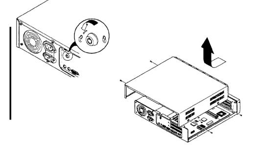
Figure 3 - 1 Unlocking and Removing the Outside Cover
