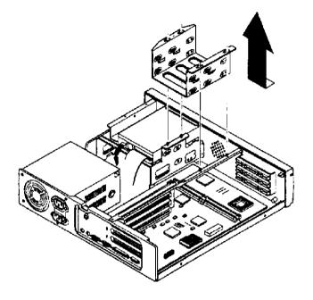
Figure 3 - 10 Removing the HDD Mounting Tray
