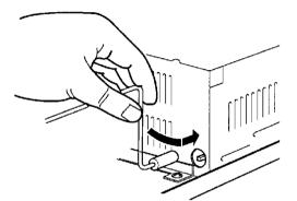
Figure 3 - 12 Pulling off Remote On/Off connector
