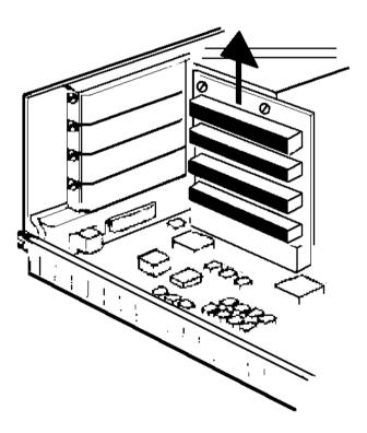
Figure 3 - 14 Installing Bus Expansion Board
