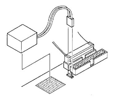
Figure 3 - 15 Disconnecting and removing the Battery
