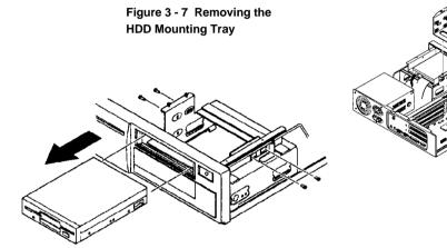
Figure 3 - 8 Removing the 3<sup>1</sup>/<sub>2</sub>-Inch FDD
