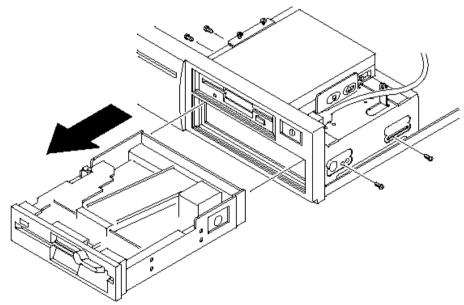
Figure 3 - 6 Removing a 51/4-Inch FDD
