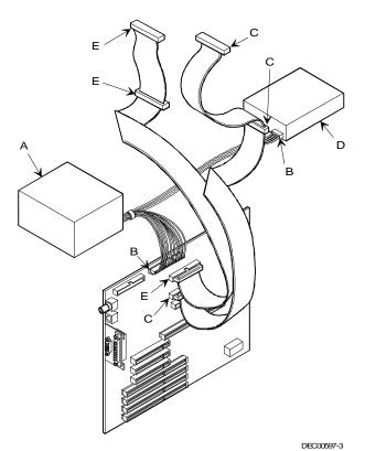
Figure 3 - 24 Primary and Secondary IDE Drive Data Cable Connections
