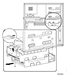
Figure 3 - 13 Removing the Lower Drive Bay Assembly
