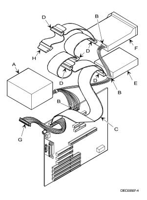
Figure 3 - 25 SCSI Cable Connections
