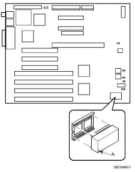
Figure 3 - 22 Replacing the Server Battery
