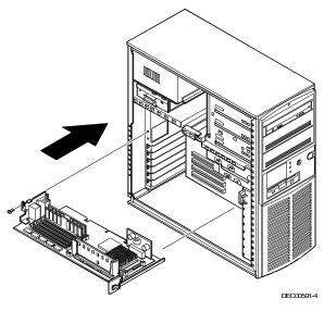
Figure 3 - 19 Upgrading the CPU Module (Pentium CPU Module Shown)
