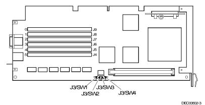
Figure 3 - 6 Pentium CPU Module Jumper Locations
