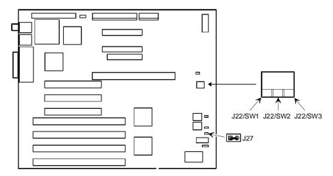
Figure 3 - 4 Main Logic Board Jumper Locations
