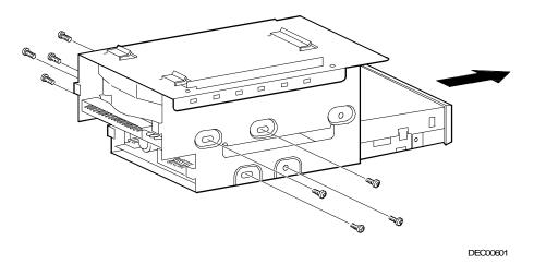
Figure 3 - 14 Removing the Lower Drive Bay Devices
