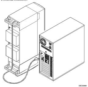
Figure 3 - 26 Connecting an External Storage Box
