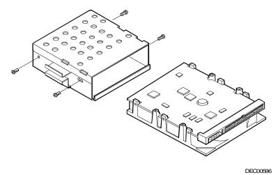
Figure 3 - 12 Removing a 31/2-Inch Device in the Rear Drive Bay Assembly
