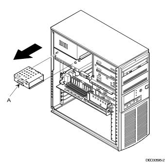
Figure 3 - 11 Removing the Rear Drive Bay Assembly
