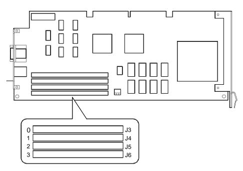
Figure 3 - 7 i486 CPU Module SIMM Socket Locations
