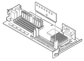
Figure 3 - 18 Installing a Secondary Cache Module
