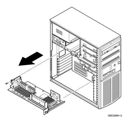
Figure 3 - 17 Removing the CPU Module (Pentium CPU Module Shown)
