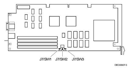
Figure 3 - 5 i486 CPU Module Jumper Locations
