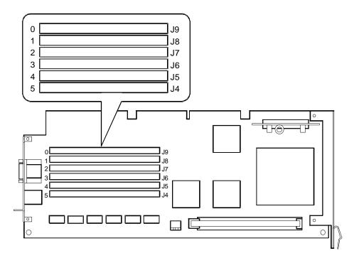
Figure 3 - 8 Pentium CPU Module SIMM Socket Locations
