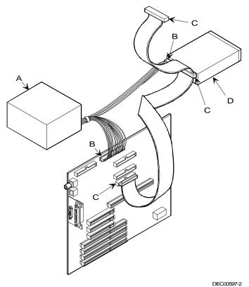
Figure 3 - 23 Diskette Drive Data Cable Connections
