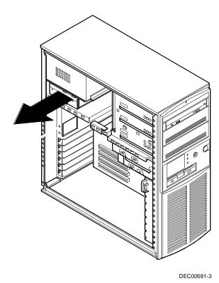
Figure 3 - 16 Removing the Power Supply
