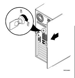
Figure 3 - 1 Unlocking and Removing the Side Panels
