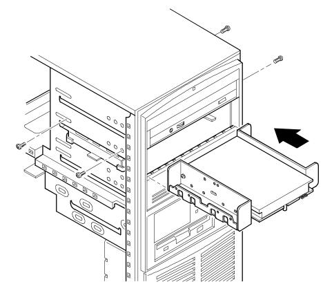
DEC00594-3 Figure 3 - 10 Removing a Device from the Second Drive Bay
