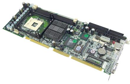
Next generation Pentium 4 processing, onboard VGA/LAN interfaces and a PCI extension connector for additional devices make the SBC-845D-VEA single board computer one of the best performing PICMG SBCs on the market.
