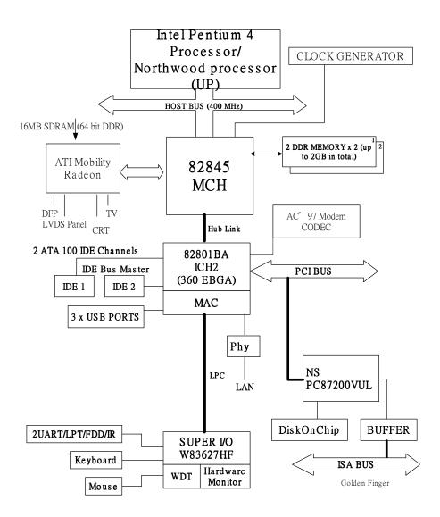
Figure 1-1. SBC-845D-VEA Block Diagram
