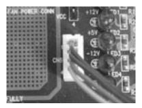
Figure 5-1. ATX power control connection on backplane
