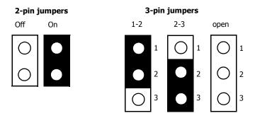
Figure 2-1. Examples of 2-pin and 3-pin jumpers
